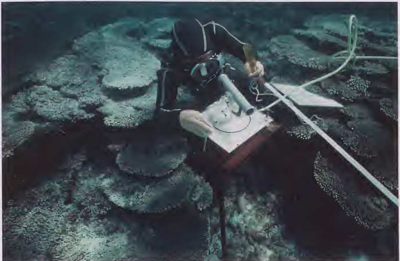
Figure 9 Surveying Zeewijk site with underwater theodolite (WA Museum © photo ZWA142).
